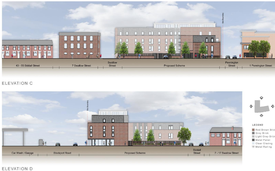
LeachRhodesWalker ARCHITECTS 8048 LAND SOUTH OF 786 STOCKPORT ROAD : COLOURED BUILDING ELEVATIONS - SHEET 2 Scale: 1:200@A2 Auth By: C.J.G. Drawn By: KM Date: 12.05.21 Dwg No: 8048_L[00]211
